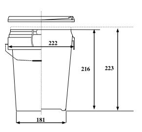
Measurements in millimetres
